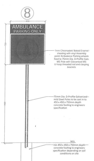
Code Ex-009 Qu. Ambulance Sign (EX-009) EX-009: Reflective Post Sign Product Description o Single Sided Post Sign 650 x 750mm on 1x P80 pole 2500mm long Graphic Details o Digital print with a UV stabiliser onto Chromadek or similar approved baked enamel sheet metal Installation guideline: 1x Post mounted 500mm into ground. Cross struts at bottom of post and concrete in hole to keep in place, as per Minimum size of concrete base to be 450 x 450 x 750mm depth Location:
