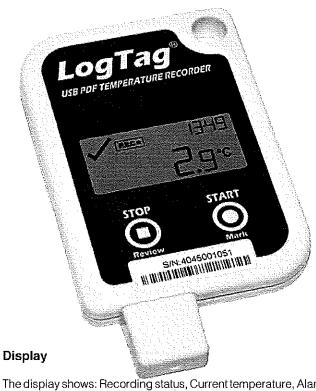
The display shows: Recording status, Current temperature, Alarm status (up to 6) and duration of any temperature excursions.
