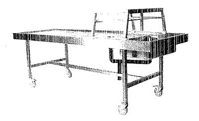
Autopsy table completely made of stainless steel AISI 304, material thickness 1,5 mm. Foundation with vertically controlled floor legs. Table top with sound attenuating foam-insulation and negative diagonal folds to the drain (Ø 50 mm). Removable perforated residual container (Ø 100 mm, height 100 mm) and PVC drain tube. Extra large organ basin (600 x 400 x 200 mm) with stand pipe, seamlessly welded, free from sharp edges and well polished.
