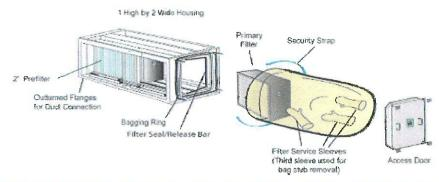
CamContain Housings are designed with safety in mind. Each housing is shipped with an instruction book detailing how to change the filters. The basics of filter change include installing the new filters in the change-out bag, securing the bag over the ribbed openings on the housing door opening, and performing the filter change entirely within the bag.
