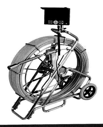
Drain/Pipe Inspection Camera that with self-leveling feature 38mm camera head, a removable 7inch LCD monitor with DVR, a 100-120m fiberglass push cable reel, all parts (including camera head, monitor, cable etc) are mounted on a robust stainless steel wheel. This system is widely used in inspections of Sewer, central air conditioning, chimney, plumbing, building, cable pipe and pipes ventilation systems and other places.
