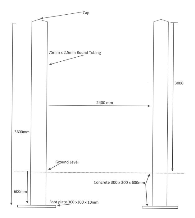
FRAME IS TO BE HOT DIPPED GALVANIZED AFTER WELDING AND DRILLING
