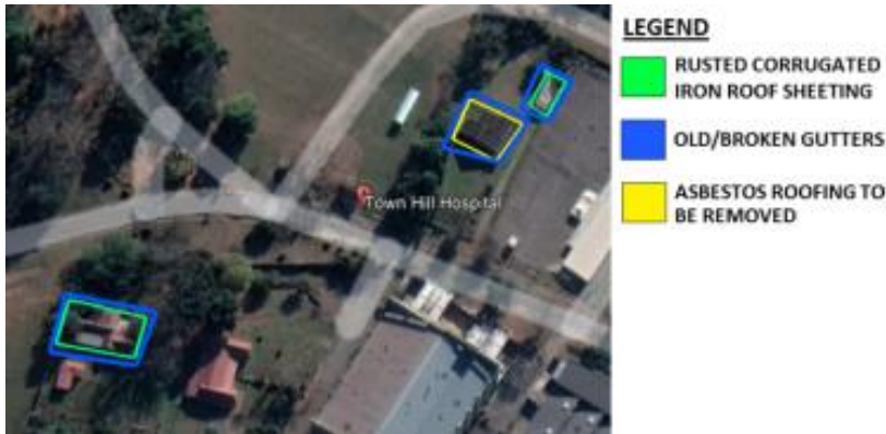
Figure 6: Site findings at residences outside the Townhill Hospital gates
