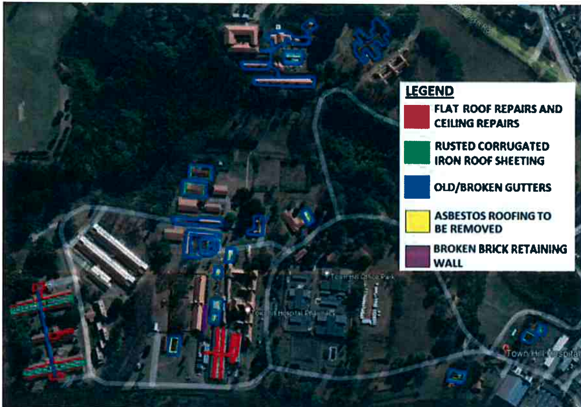
Figure 4-1: Townhill Hospital Buildings and identified sections with problems
