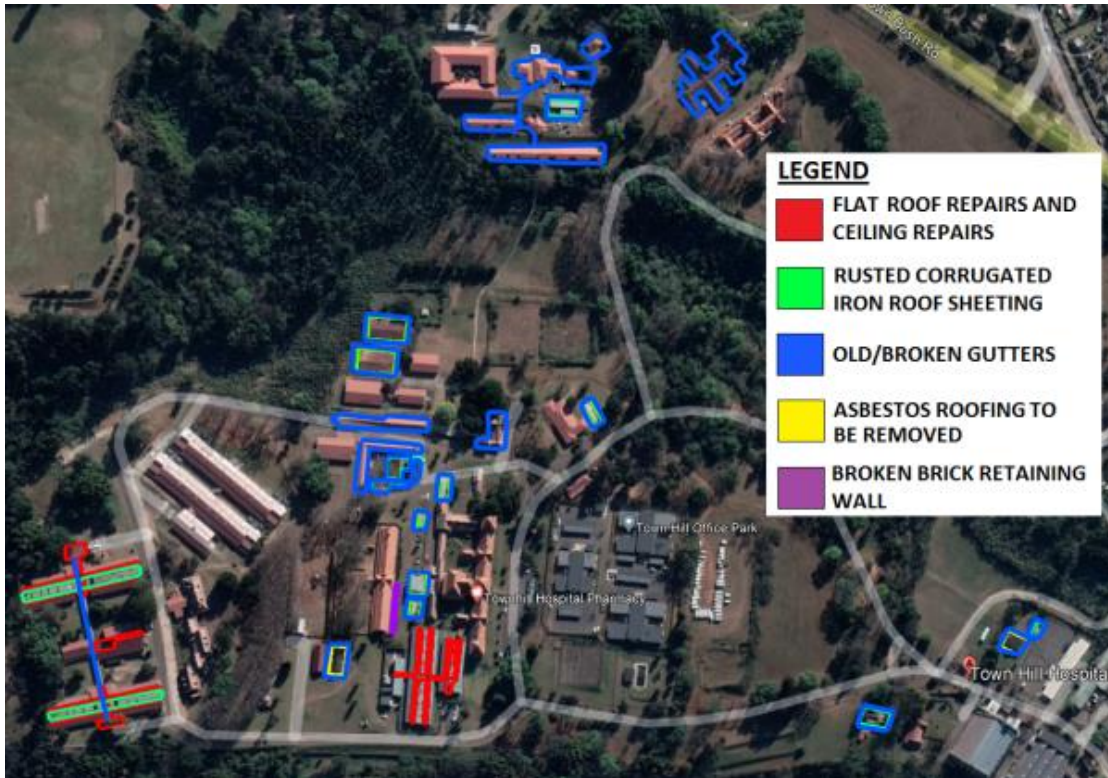
Figure 1: Townhill Hospital Buildings and identified sections with problems
