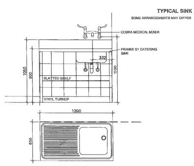
FRANKE MODEL "S1" 1200x650 CATERING SINK SINGLE END BOWL MANUFACTURED FROM GRADE 304 18/10 STAINLESS STEEL 11.2mm THICK WITH 150mm HIGH INTEGRAL SPLASHBACK TO THE REAR AND 50X10mm TURN DOWN WITH BEADED EDGE TO REMAINING SIDES WITH 500x500x230 PRESSED BOWL AND 40mm WASTE OUTLET COBRA 309-40 ANTI-THEFT CHROME PLATED PLUG
