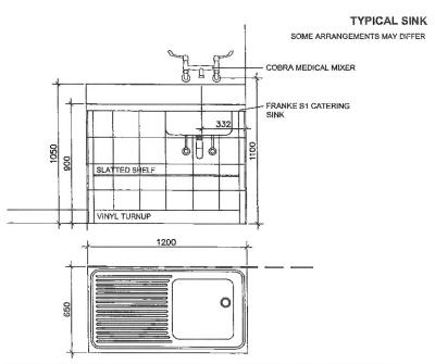
FRANKE MODEL \*S1\* 1200x650 CATERING SINK SINGLE END BOWL MANUFACTURED FROM GRADE 304 18/10 STAINLESS STEEL 11.2mm THICK WITH 150mm HIGH INTEGRAL SPLASHBACK TO THE REAR AND 50X10mm TURN DOWN WITH BEADED EDGE TO REMAINING SIDES WITH 500x500x230 PRESSED BOWL AND 40mm WASTE OUTLET COBRA 309-40 ANTI-THEFT CHROME PLATED PLUG
