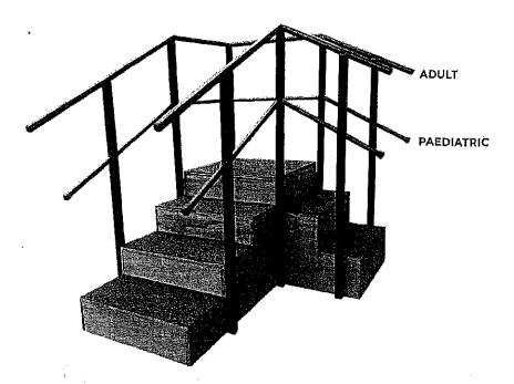
Sturdy 90° medical stairs used for Gait Rehabilitation training. Manufactured with solid wood, Carpeted non-slip surface. Powder coated metal height adjustable hand (grab) rails. The handralls are height adjustable from 40 to 90cm with locking pins and bolts. The one side is comprised of 4 steps with a height of 15cm each, the opposite side is comprised of 3 steps with a height of 20cm each.
