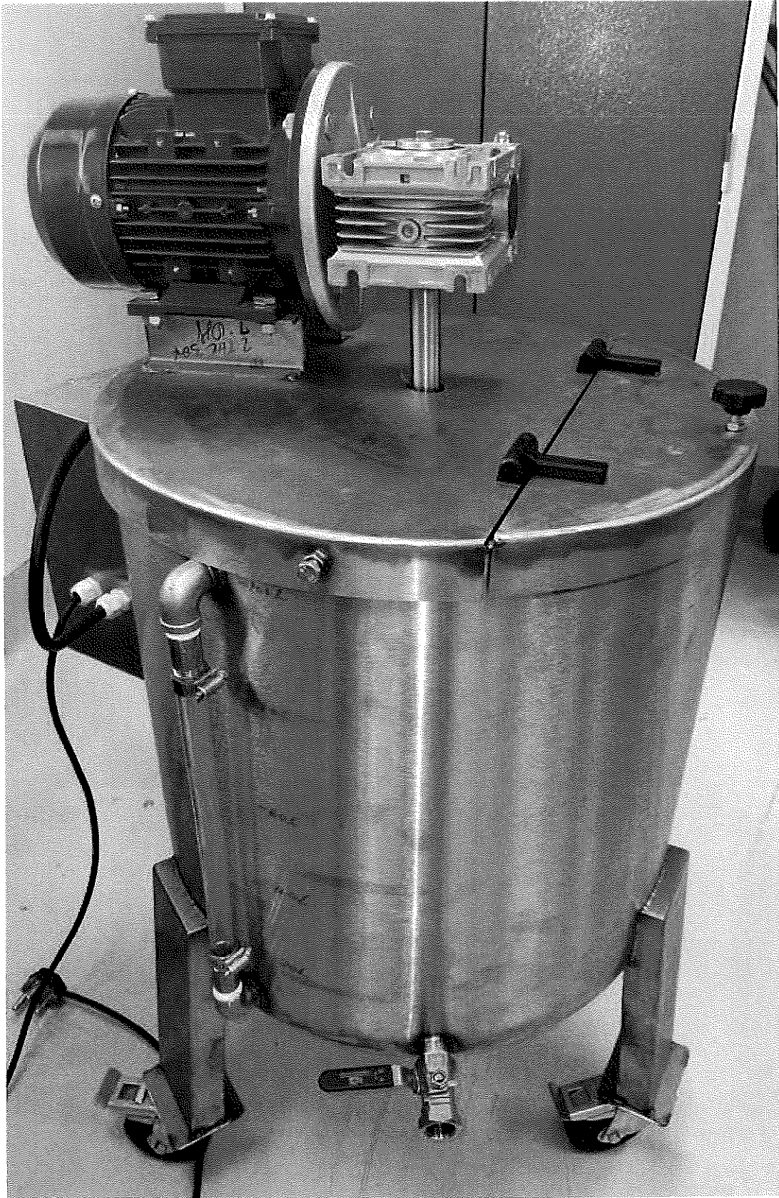
Pharmacy manufacturing drum to be refurbish/modified by installing counter weight
