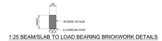
1:25 BEAM/SLAB TO LOAD BEARING BRICKWORK DETAILS
