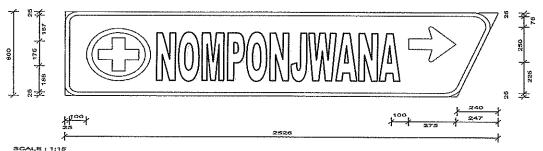
SCALE: 1:15 RADII ON RIGHT: 100 mm OTHER RADII: 75 mm BORDER COLOUR: WHITE CLASS: 1 PANEL COLOURS AND ARROW TYPES STACK TOP BACKGROUND: BROWN CLASS: 1 ARROW TYPE: 1
