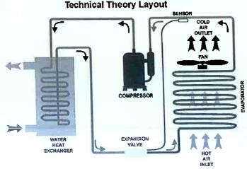
When a heat pump is used for heating, it employs the same basic refrigeration-type cycle used by an air conditioner or a refrigerator, but in the opposite direction — releasing heat into the conditioned space rather than the surrounding environment. In this use, heat pumps generally draw heat from the cooler external air or from the ground.
