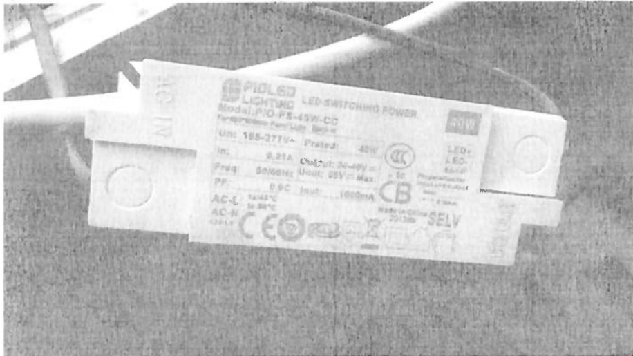
LED light power supply: PIO-PS-40W-cc
